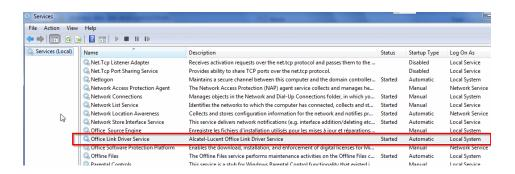
Note: In case of a PC crash while the OHL driver is running, the driver restarts automatically only if it has been installed as an automatic "start up type" in Windows "Services" (this is the case by default after installation).
